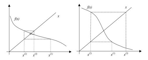
Figure 2.7. Converging (left) and diverging (right) iterations.
